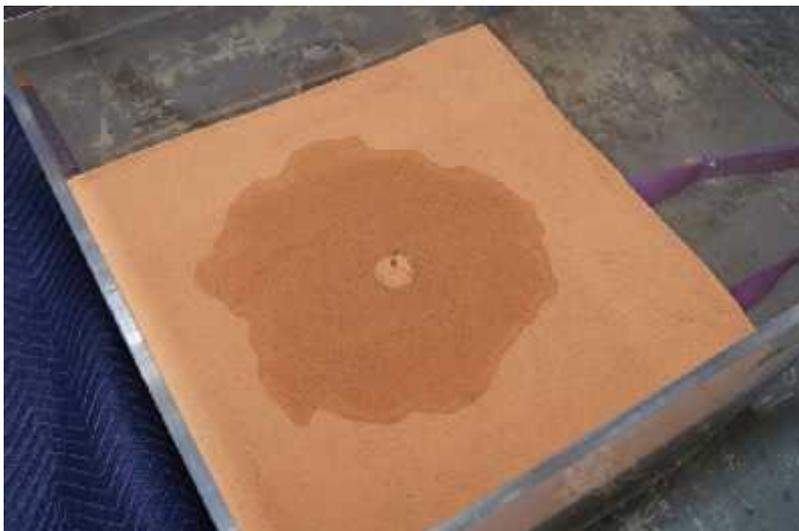
Figure 16 wetted pattern at the drip point of the control
