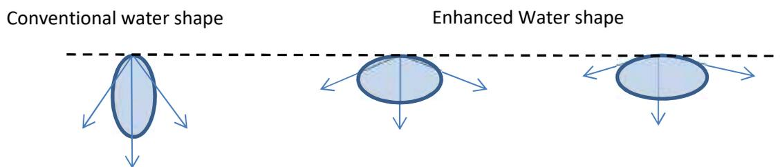
In the control, the primary capillary activity is in the downward thrust, whereas in the treatment this changes significantly to flatten the water ball.
