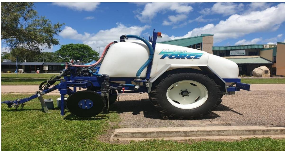
*Figure 2: Liquaforce applicator that allows for precise application of product in a narrow band at the stool.*
